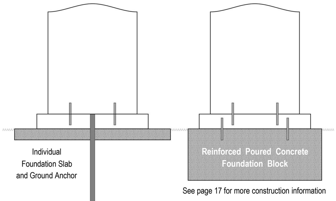
Fig 10 ~ Pillar Foundation using threaded dowels (Studs) and 75mm (3") granite (2'3"x1'9")
