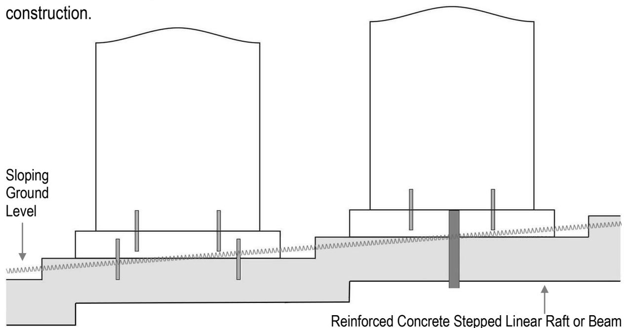
*Note: It is recommended that a Burial Authority uses the services of an appropriately qualified specialist to produce a design and specification for all Cast-in-Situ foundations.*
