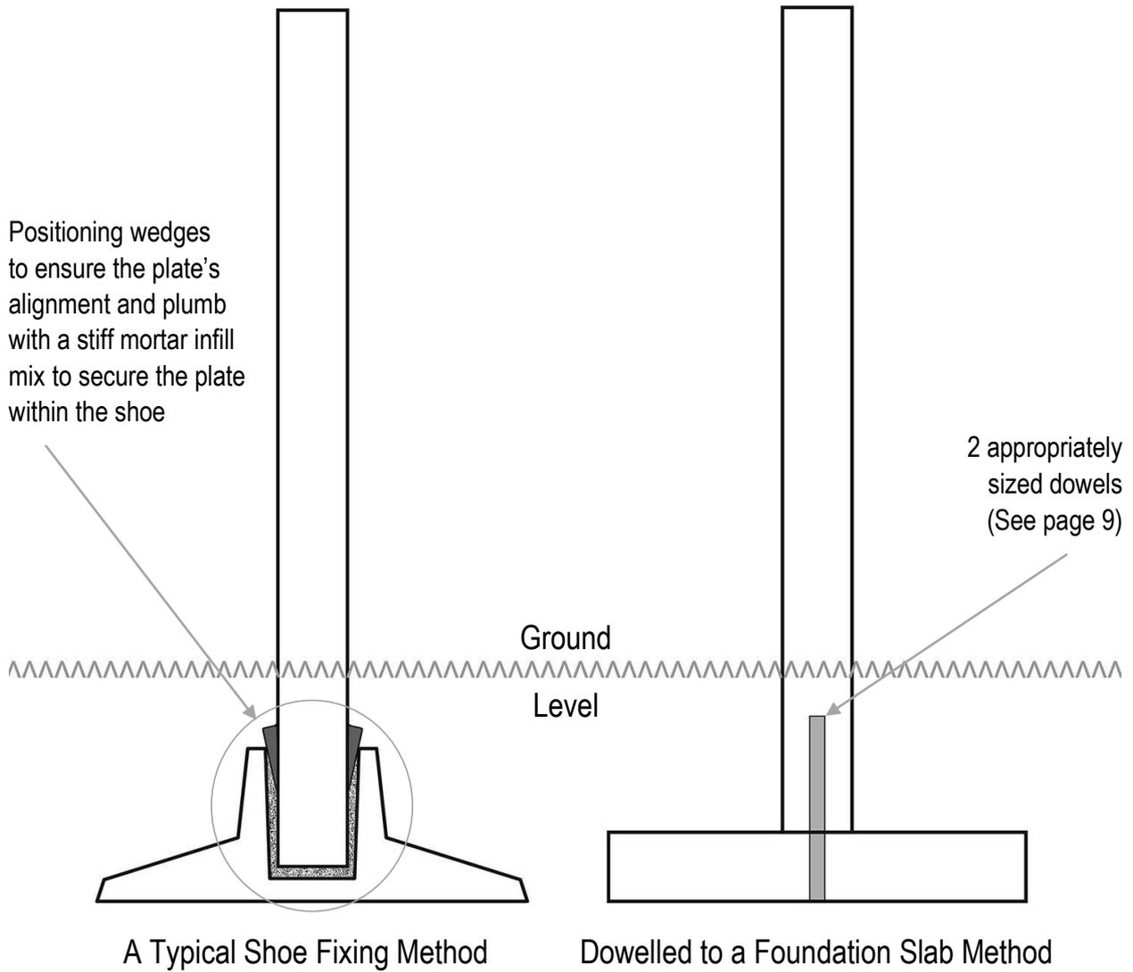
The minimum depth below ground is 375mm (15") or 25% of the overall height (including the foundation) whichever is greater.
