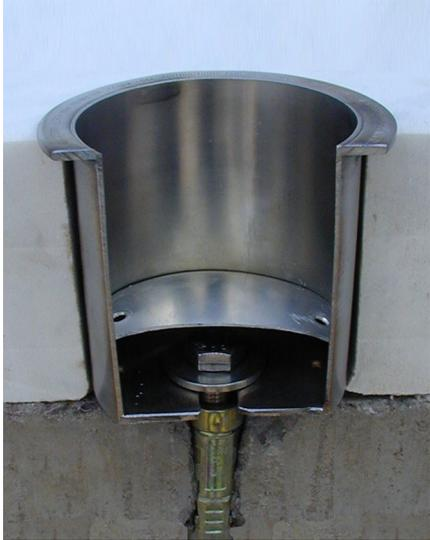
The Lockdown System comprises a stainless steel flanged sleeve which fits inside a standard flower container hole. An expansion bolt inserted through a hole in the base of the sleeve locks the memorial down to the foundation. No cement is required. A normal flower container fits inside the sleeve for flowers. To remove the memorial for further work it is simply a case of undoing the bolt.
